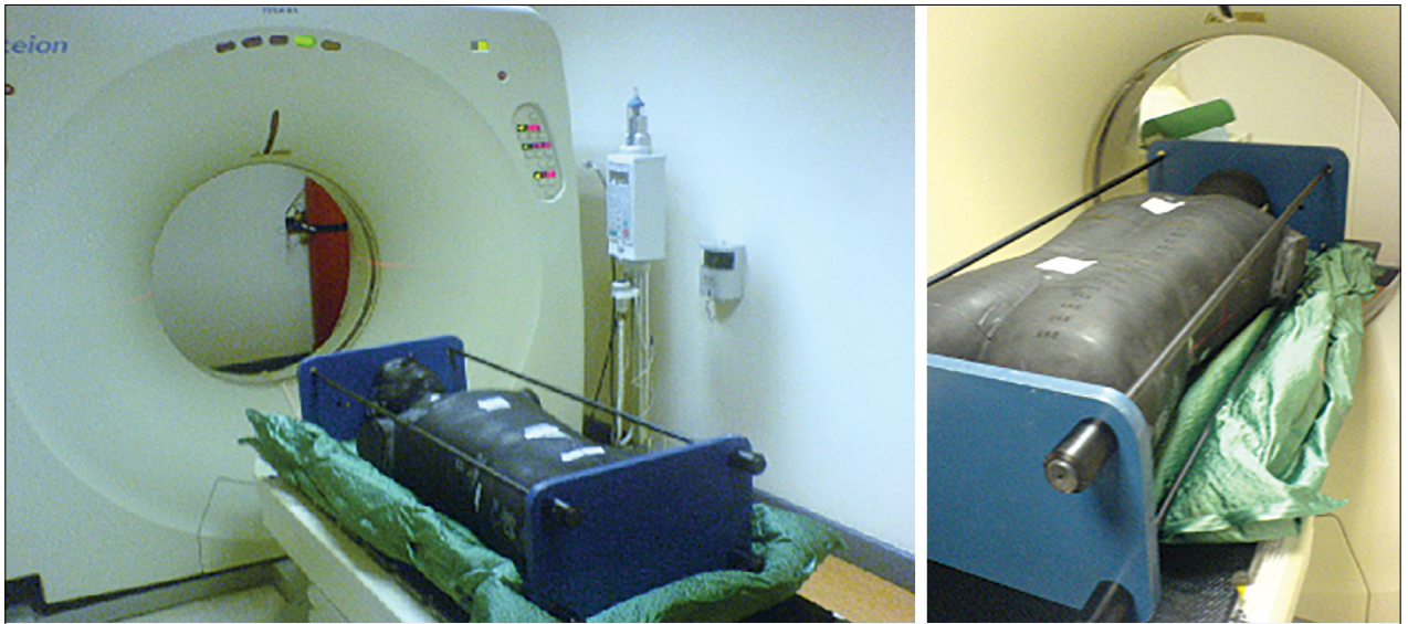
Fig. 1. Rando Phantom supine and prone position with vacuum bed.
